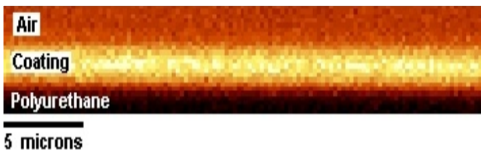
Fig. 4: Raman cross sectional image of a coating on a polyurethane catheter.
